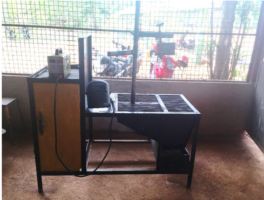
Figure 3 Movable Welding Table with Positioner and Waste Catch Basin
